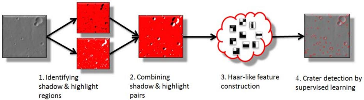
**Figure 1: Diagram illustrating the crater-detection framework. (1) Crescent-like shadow and highlight regions are identified. (2) Shadow and highlight regions that can be matched are used to construct crater candidates. (3) Haar-like features are calculated using 9 kernels on crater candidates. (4) Craters are identified using supervised learning.**
