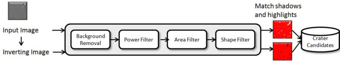
Figure 3: Diagram illustrating individual steps in constructing crater candidates
