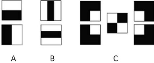
**Figure 4: 9 rectangle features: (A) 2 two-rectangle features, (B) 2 three-rectangle features, (C) 5 four-rectangle features.**
