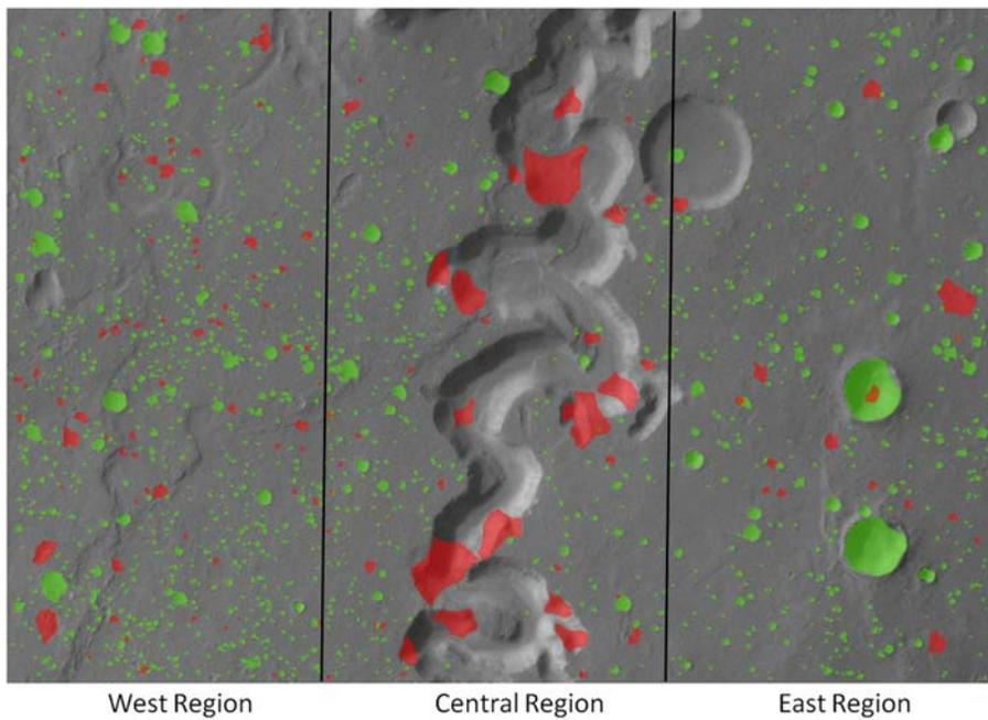
Figure 10: Craters ( $\leq 5000$ -meter in diameter) detected in a  $37,500 \times 56,250 m^2$  test image. (Best viewed in color.) Green: True detections, Red: False detections.
