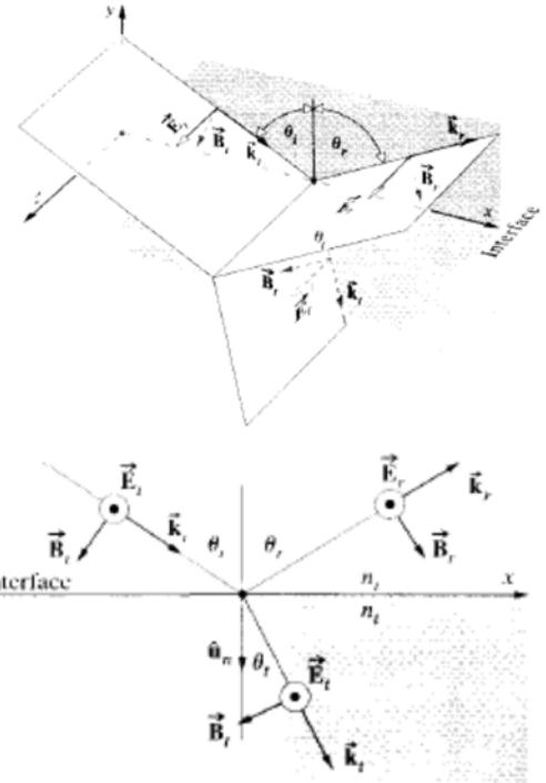
The electric field may lie in the plane of incidence or be parallel to it. Here are the figures from Hecht that show this case. For this case, the magnetic fields have all been selected to have the same direction, consistent with  $\mathbf{E}$  and  $\mathbf{k}$ . This time, we apply the same BCs, but the equations are different because the electric has been rotated by 90 degrees.
