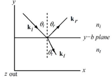
So long as  $\mathbf{E}$  is perpendicular to  $\mathbf{B}$  and  $\mathbf{k}$ , we are OK. It turns out that Maxwell's equations make some interesting conditions on  $\mathbf{E}$  and  $\mathbf{B}$  at an interface. They are most easily used in integral form to derive what are called boundary conditions. Here are the boundary that apply when an EM wave crosses a dielectric boundary.
