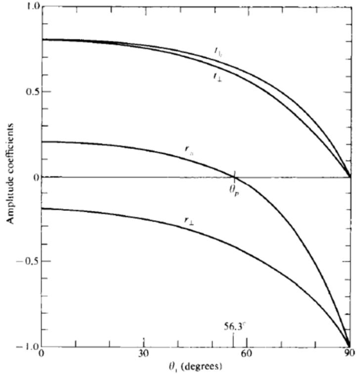
These are the reflection coefficients only because the transmission coefficients do not show any particularly interesting behavior. Note that for an internal reflection,  $r_{\perp}$  is always positive, but the parallel coefficient changes from negative to positive at the polarizing angle.
