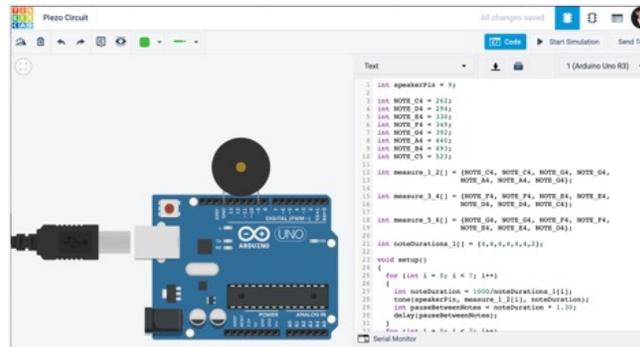
The activity is done using the online tinkercad interface (an Arduino simulator), the Arduino components are shown on the left, coding on the right. The frequency values need to be recalculated for each piece. Once everything is ready to go, students will click on the 'Start Simulation' button to hear what they've created.
