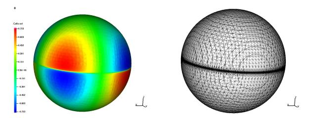
Figure 13: Numerical solution and the Shishkin mesh for the advection-diffusion problem from Example 6 with the  $Pe = 10^4$ .
