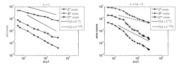
Figure 9: Decrease of the error in the  $L^2(\Gamma)$ ,  $H^1(\Gamma)$  and  $L^{\infty}(\Gamma)$  norms for the advection-diffusion problem from Example 6 with Pe = 1 (left) and Pe = 100 (right). The problem is solved on a sequence of adaptively refined grids.
