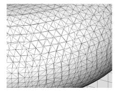
Figure 1: Left: A cutaway of a bulk domain shows the bulk octree mesh three times refined towards the surface and the resulting approximate surface  $\Gamma_h$  for the part of a torus. Right: The zoom-in of the resulting surface triangulation. The triangulation does not satisfy a minimal angle condition.
