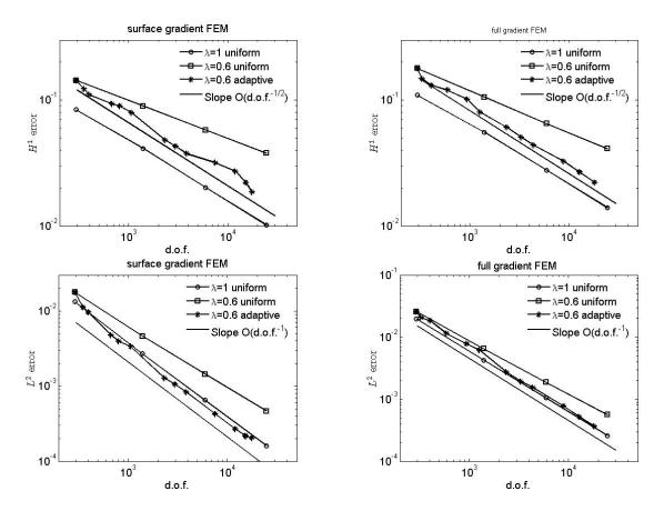
Figure 7: Decrease of the error in  $H^1(\Gamma_h)$ -norm (upper plots),  $L^2(\Gamma_h)$ -norm (bottom plots) for the adaptive algorithm and Example 5. Left column plots show results for the surface gradient formulation (14), while the right column plots show results for the full gradient formulation (16).
