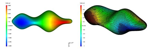
Figure 4: Illustration of the surface and solution from Example 3. The right figure shows also triangulation after 7 steps of adaptation based in the error indicator.
