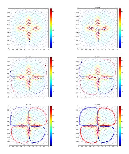
Fig. 4.5. Velocity field and motion of four L-shaped enantiomers (two left-handed and two-right-handed) initially placed in the middle between two counterrotating vortices
