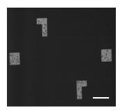
Fig. 4.1. Schematic representation of the fabrication of photoresist particles (left) and microparticles of different shapes still attached to the silicon wafer. The scalebar represents  $300\mu m$  (right).
