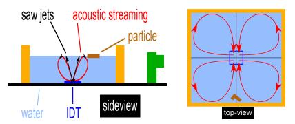
Fig. 1.3. Left: Schematic sideview of the experimental setup. Right: Topview of the vorticity pattern created at the fluid surface.
