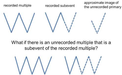
Figure 1: Using a recorded multiple to find an approximate image of an unrecorded primary of the multiple: illustrate the need to remove unrecorded multiples. A solid line ( — ) is a recorded event, and a dashed line ( - - - ) connotes an unrecorded event.
