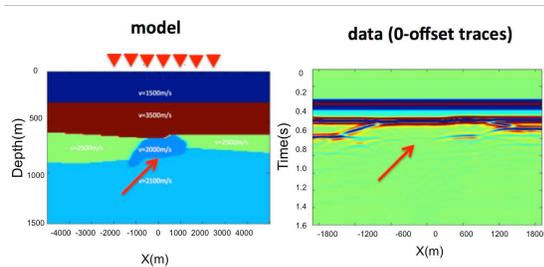
Figure 4: *The model and zero offset traces of data. The base salt is almost invisible because the primary generated by the base salt is negatively interfering with an internal multiple.*
