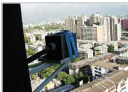
Figure 2 - HONO measurements at high-rise building in Santiago de Chile at 53 m (lower picture). UH student, Giovanna Croxatto (now at University of Copenhagen) checking the LOPAP system (picture above)
