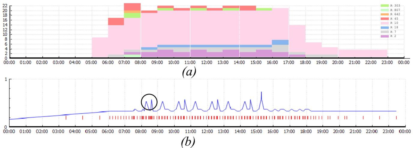
Fig. 6: (a) the bus services provided at a user selected stop. Different color blocks show the numbers of buses of the respective routes that provide services at the stop. (b) the service overlap function at a selected stop.
