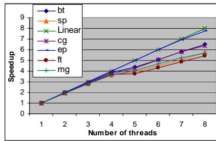
Fig. 9. Speedup of SPEC OMPM2001 on Sun Fire V490
