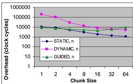
Fig. 7. Scheduling overhead on Dell Precision 450
