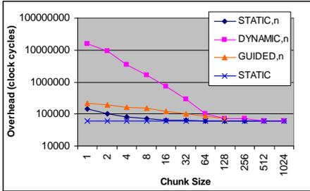
Fig. 3. Scheduling overhead on Sun Fire V490
