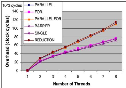
Fig. 1. Synchronization overhead on Sun Fire V490
