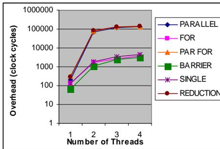
Fig. 5. Synchronization overhead on Dell Precision 450
