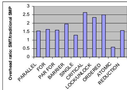
Fig. 8. Synchronization overhead ratio: SMT vs. traditional SMP
