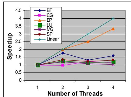
Fig. 11. Speedup of SPEC OMPM2001 on Dell Precision 450
