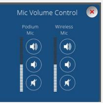
The "Mic Volume" controls the volume for the podium microphone and the wireless microphone.
