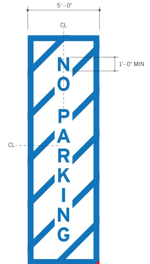
**SIGN TYPE - ADA Parking Zone Clearance Pavement Marking**
