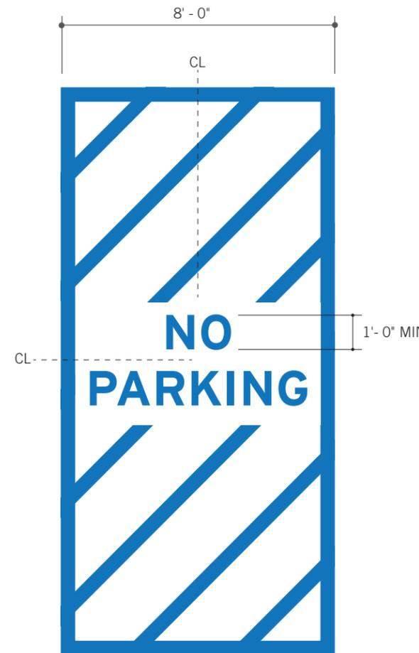
**SIGN TYPE - ADA Parking Zone Van Clearance Pavement Marking**
