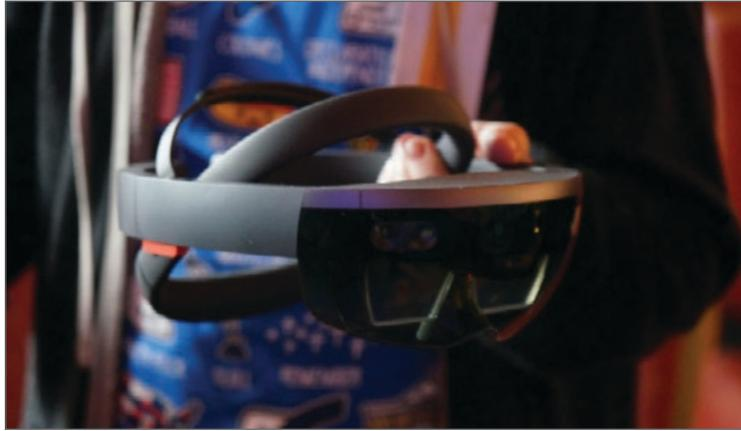
The programs are being developed primarily for the Microsoft HoloLens, an augmented reality headset that places holograms and information over the physical world, said computer science professor Chang Yun. Some, however, are made in virtual reality using the HTC Vive.
