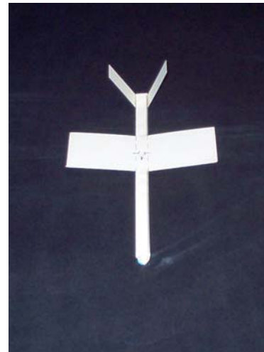
Front view showing the “V” tail and triangular prism fuselage.
