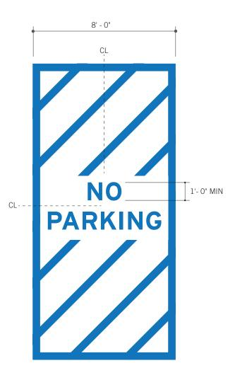
SIGN TYPE - ADA Parking Zone Van Clearance Pavement Marking Scale: 1/4" =1'
