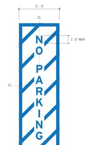
**SIGN TYPE** - ADA Parking Zone Clearance Pavement Marking Scale: 1/4" =1'
