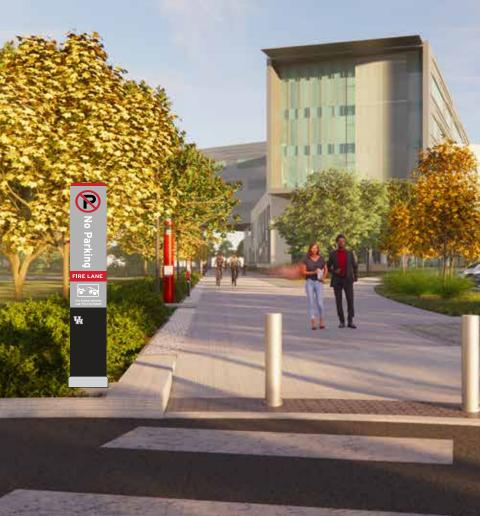
NOTE: Provide fire lane marker and removable stainless steel bollards at entrances to combined pedestrian walks/fire lanes
