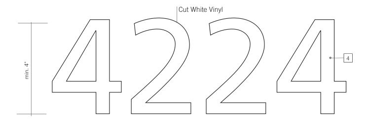
**SIGN TYPE Q3** - Building Address - Masonry Application
