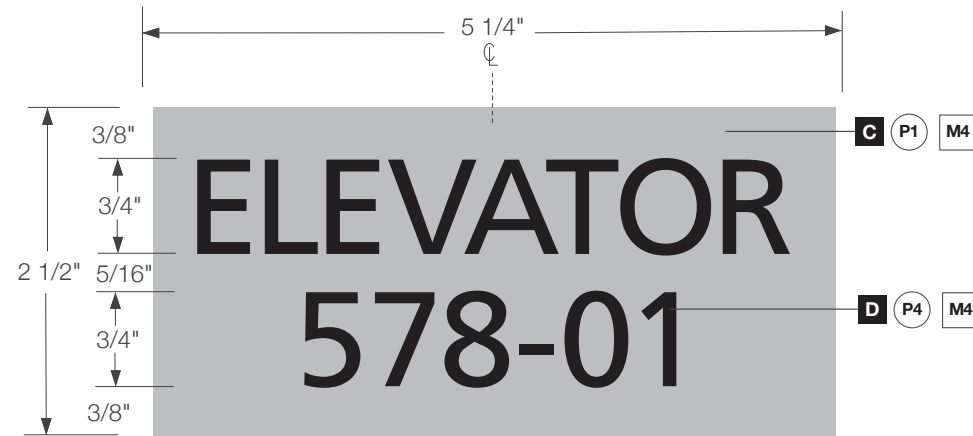
E7 Elevator Identification Plaque
