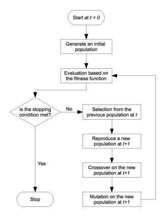
Figure 11.5.1: The Structure of the Genetic Algorithm Process
