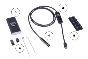
Figure 2 – WiFi equipped camera (1) 3 mm camera with stiff cable, (2) dimmer switch for lights, (3) micro-WiFi transmitter, (4) camera accessories including right-angle mirror, (5) suction cup sleeve for mounting the micro-WiFi
